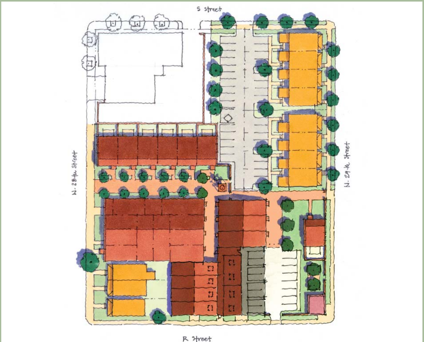
master plan showing existing warehouses converted to lofts, new infill for townhouse fabric, and new retail
